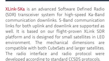
The Ka-Band transmitter provides very high downlink data rates of up to 200 Mbps. Supported modulation schemes include BPSK, QPSK and higher order modulations with appropriate FEC coding schemes. Adaptive Modulation and Coding (AMC) schemes are applicable to maximize data throughput.
